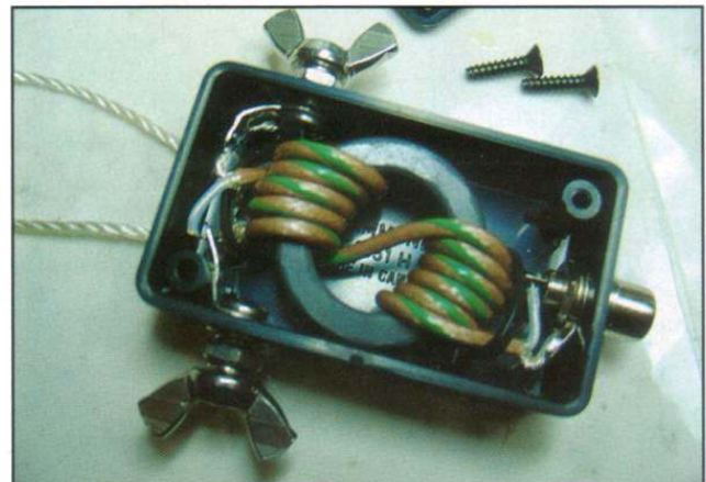
Photo D— The balun (see text) performs double duty, helping minimize RF "bites" in areas with poor or no ground, and providing a center support and feedline connection point for the antenna.
